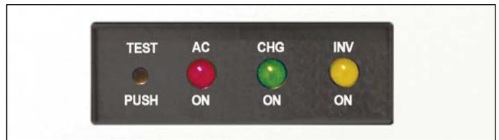
All LPS systems provide a monitoring panel on the front of the unit to show operating status at all times. The panel provides a test switch for user initiated system tests and a 3-LED array that provides an intuitive visual indication of unit readiness.
